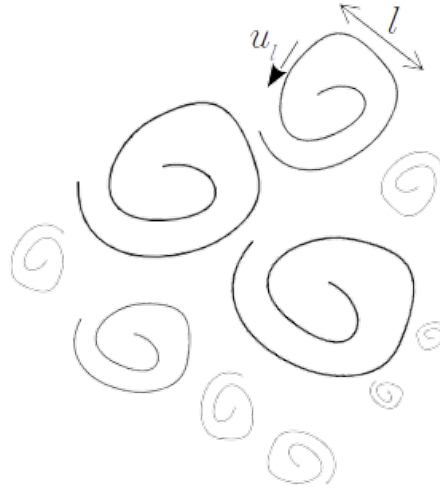
Figure 1.3: Eddies: smaller and smaller patterns are generated as energy cascades down from the larger to the smaller scales
